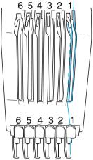
Wind the thread clockwise once around the number 1 thread tension disc.
